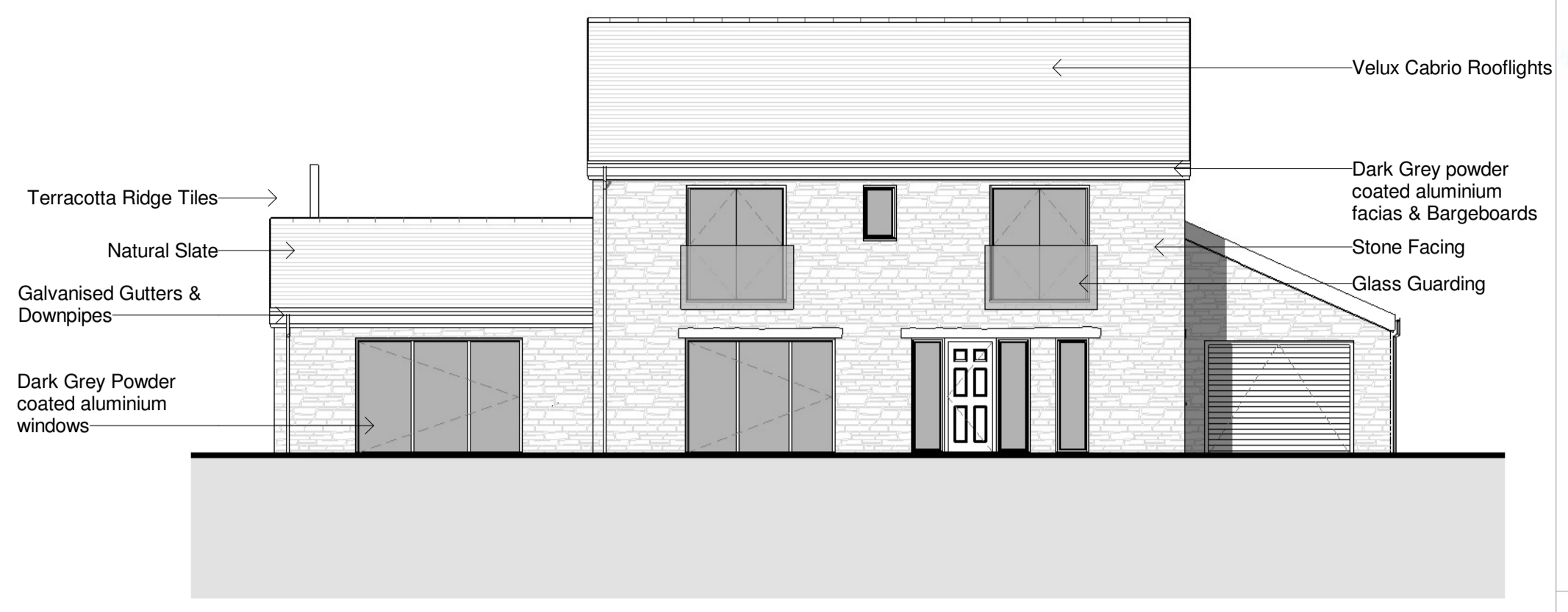
3 South Elevation 1 : 100
